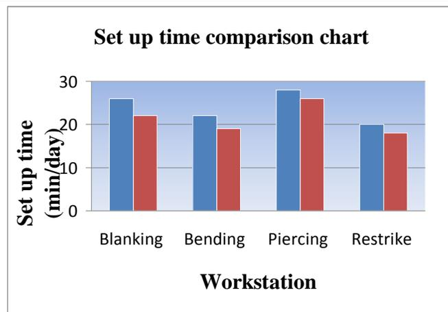
Fig. 3. Set up time comparison.
